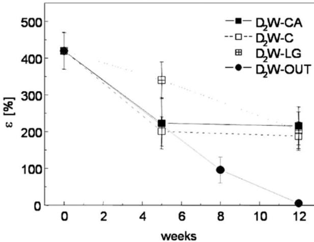
Fig. 7: Relative elongation at breaking  $\epsilon$  [%] of the individual types of D<sub>2</sub>W samples.
