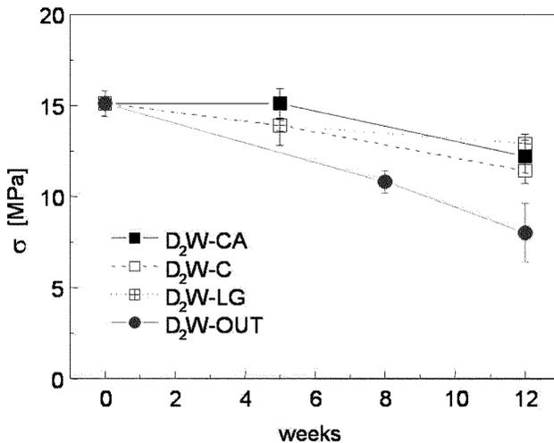
**Fig. 5:** Tensile strength  $\sigma$  [MPa] of the individual types of  $D_2W$  samples.
