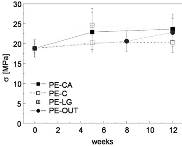
Fig. 6: Tensile strength  $\sigma$  [MPa] of the individual types of PE samples.
