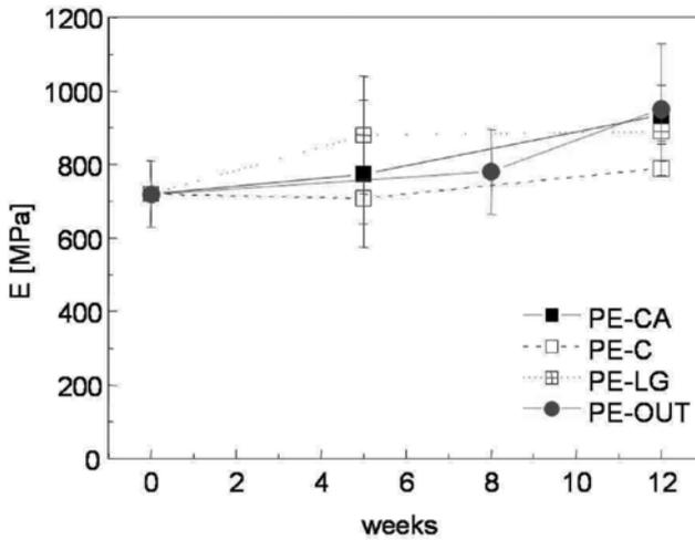
Fig. 10: Elastic modulus E [MPa] of the individual types of PE samples.
