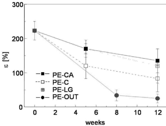
Fig. 8: Relative elongation at breaking  $\varepsilon$  [%] of the individual types of PE samples.
