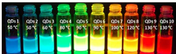
Fig. 1 Colour of QDs was observed in the transilluminator (excitation: 312 nm) and whole visible light spectrum was observed.
