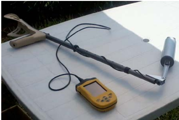
Fig. 1 Prototype of the handheld sensor for simultaneous measurement of NDVI and NRERI indices. The instrument consists of measuring optical head with filters and detectors, small portable computer and a support rod with a joint mechanism to ensure the vertical position of the sensor
