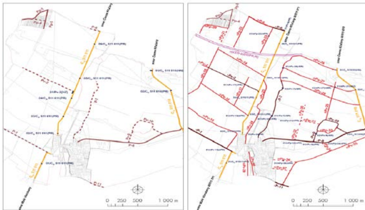
Fig. 2: Reconnaissance of existing field road in project perimeter (left), new design of transportation facilities and measures in the project's perimeter (right)
