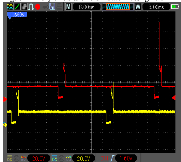
Fig. 6 Primary circuits of distributor-less ignition
