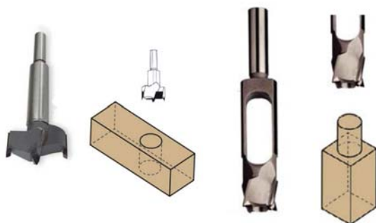
Fig. 1 Joint production scheme: (left) forstner drill bit – mortise, (right) plug cutter bit – tenon
