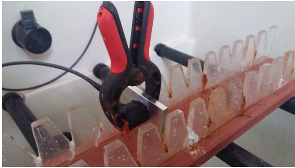
Figure 1 The insertion of the sample to corrosion chamber
