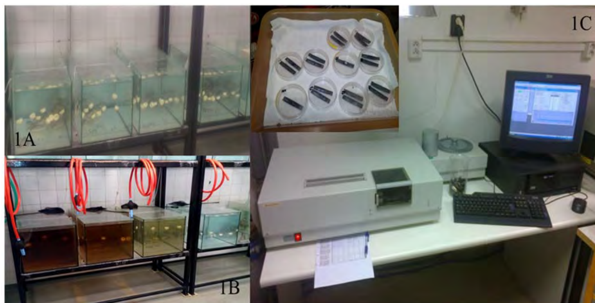
Figure 1 The glass fish tanks with sodium chloride (A), the glass fish tanks with humic acid (B), atomic absorption spectrometer AMA 254 (C)
