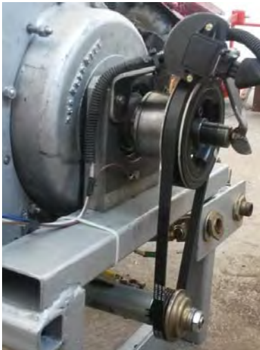
Figure 3 Load setting mechanism of the hydrodynamic brake with the feedback
