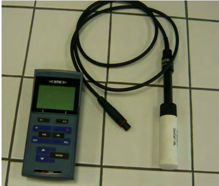
Figure 1 Measuring device Multi 3320 and sensor 325 CelloX ® in a calibration vessel OxiCal ® SL
