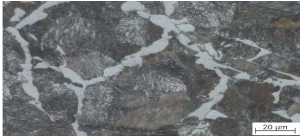
Figure 5 Detailed structure of the basic material steel STN 12050
