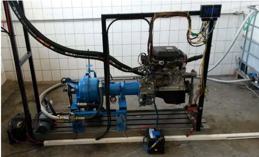
Figure 1 Hydrodynamic brake with mounted an internal combustion engine
