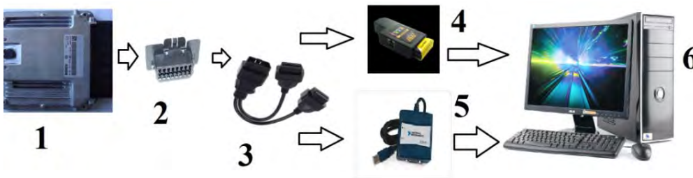
Legend: 1 – ECU EDC17CP20, 2 – OBD connector, 3 – OBD reduction; 4 – Multiplex 7I, 5 – CAN BUS converter, 6 – PC
