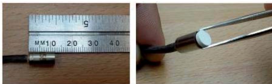
Figure 3 Pore Pressure Transducer (Druck PDCR81), fitted with a high air entry value porous disc.
