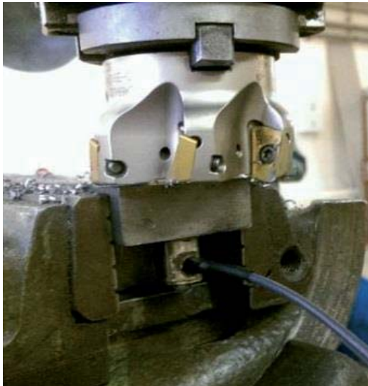
Figure 1 Cutter with indexable inserts – Place the piezoelectric sensor on the sample
