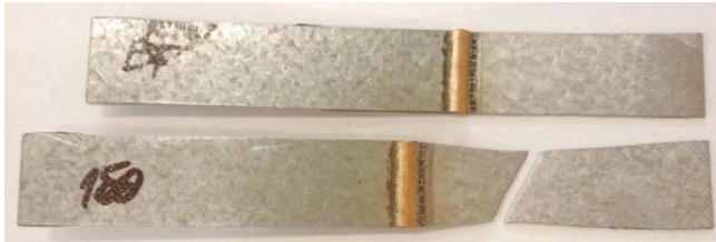
Figure 3 Specimen before and after tensile strength test
