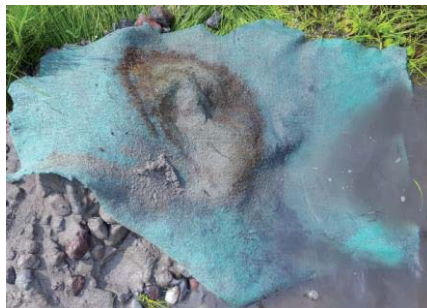
Figure 2 The tested nonwoven geotextile after exploitation in the Białobrzegi earthfill dam
