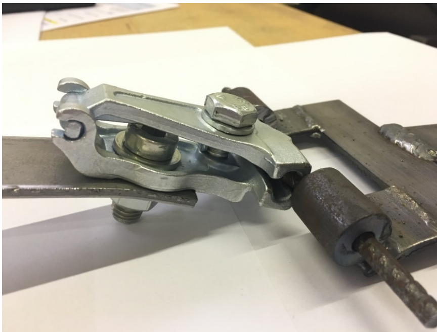
Figure 6 Deformation of the tested clamp
