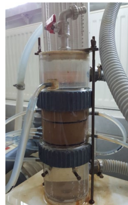
B) Nonwoven geotextile and soil
