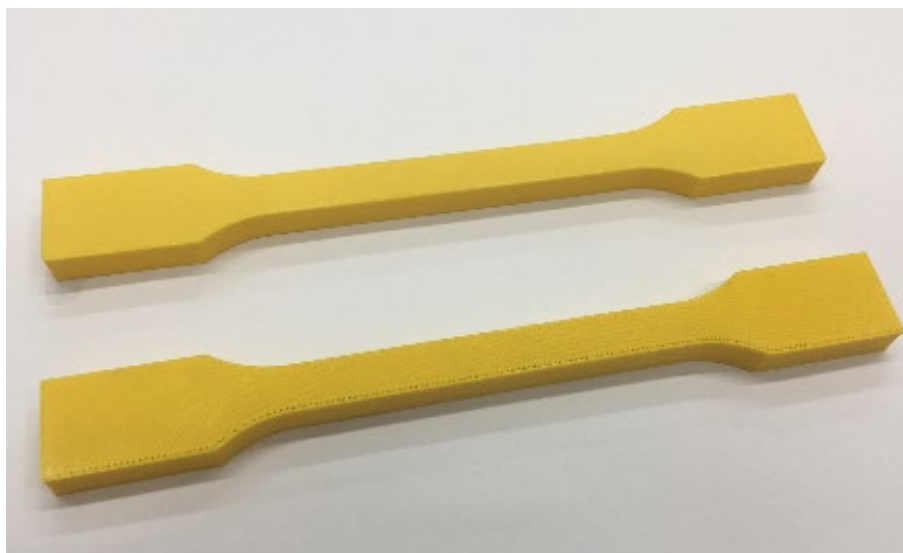
Figure 1 Tested specimens according to ČSN EN ISO 527
