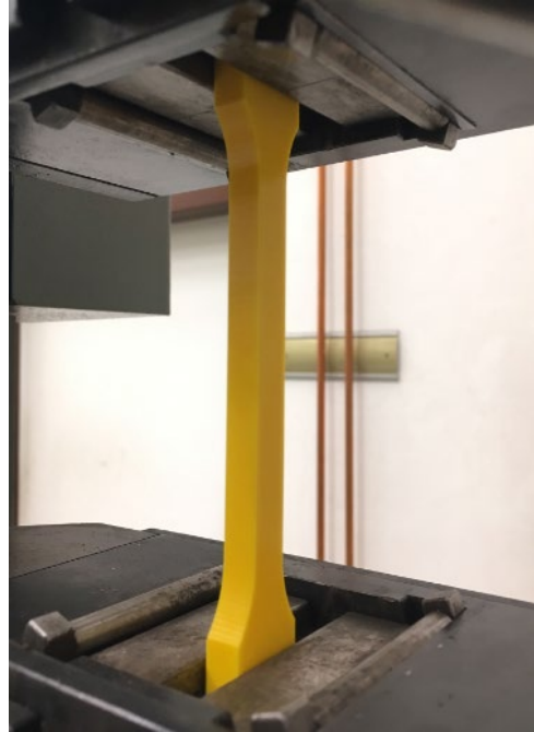
Figure 3 Sample clamped between jaws of testing device
